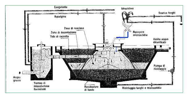
4. Type of clarification process: Cyclofloc<sup>TM</sup>
